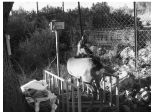
Plate 2. A standard sheep scale was modified for Roe deer Capreolus capreolus . The modification includes removing the usual cage structure commonly used for sheep and shaping the scale in such a way as to allow the Roe deer to jump off at will. A. Wallach.
